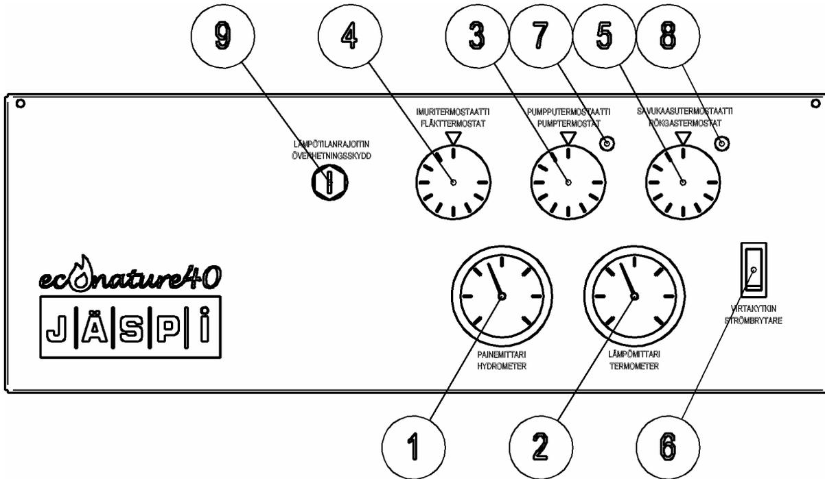
1. **Pressure gauge.** Measures pressure in the boiler.
